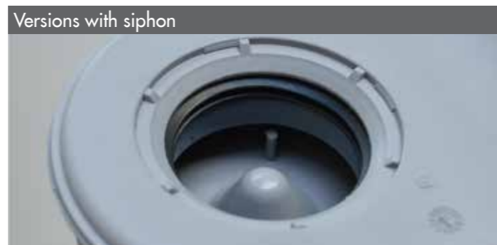
You do not need to glue the drain pipe of the channel to the siphon, because the connector provides a sufficient hold, but BE CAREFUL not to pinch the siphon's gasket when interlocking to avoid small water leaks.
