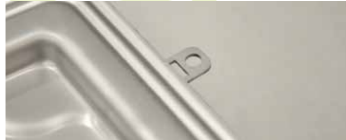
If the project manager deems it appropriate, the channel may be grounded. It has a small perforated tab, that can be bent downwards to connect the grounding.
